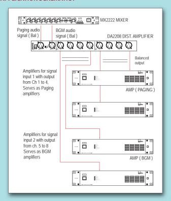
The above illustration is for Uninterrupted Paging setup. In normal setup with single input, use the link switch to form 1 input 8 outputs configuration. Each output from DA2208 can be linked up to 6 power amplifiers.
